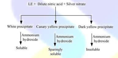
Chemistry of the test: In the Lassaigne's test for halogens in an organic compound, the sodium fusion extract is acidified with nitric acid and then treated with silver nitrate.
