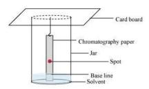
phase to different heights. The paper so obtained (shown in the given figure) is known as a chromatogram.
