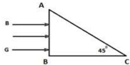
(Hint Calculate the critical angle for each and if the angle of incidence on the surface AC is greater, then TIR will take place.)
