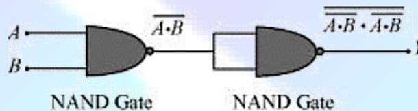
Hence, the output of the combination of the two NAND gates is given as:
