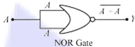
Output,  $Y = \overline{A + A} = \overline{A}$
