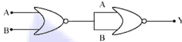
(Hint:  $A = 0, B = 1$  then  $A$  and  $B$  inputs of second NOR gate will be 0 and hence  $Y=1$ .)
