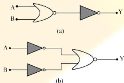
**Ans.** A and B are the inputs and Y is the output of the given circuit. The left half of the given figure acts as the NOR Gate, while the right half acts as the NOT Gate. This is shown in the following figure.
