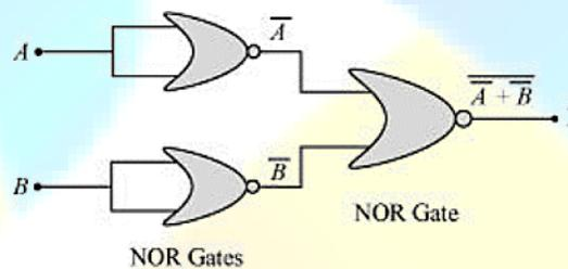
$\overline{A}$  and  $\overline{B}$  are the inputs for the last NOR gate. Hence, the output for the circuit can be written as:
