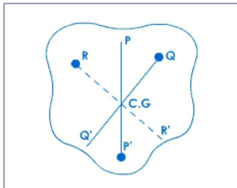
Suspend a plumb line from P and mark the position PP' on the lamina.
