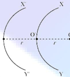
X'Y' can be considered as a virtual reflected ray for the plane mirror. Hence, a point object placed in front of the plane mirror produces a virtual image whose distance from the mirror is equal to the object distance (r).
