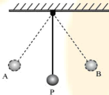
When a pendulum moves from its mean position P to either of its extreme positions A or B, it rises through a height  $h$  above the mean level P. At this point, the kinetic energy of the bob changes completely into potential energy. The kinetic energy becomes zero, and the bob possesses only potential energy. As it moves towards point P, its potential energy decreases progressively.
