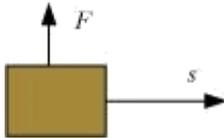
In this case, the direction of force acting on the block is perpendicular to the displacement. Therefore, work done by force on the block will be zero.
