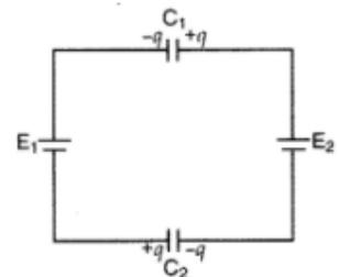
**Q.7.** Determine the potential difference across the plates of the capacitor ' $C_1$ ' of the network shown in the figure. [Assume  $E_2 > E_1$ ]
