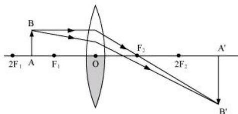
**10.** An object 5 cm in length is held 25 cm away from a converging lens of focal length 10 cm. Draw the ray diagram and find the position, size and nature of the image formed.
