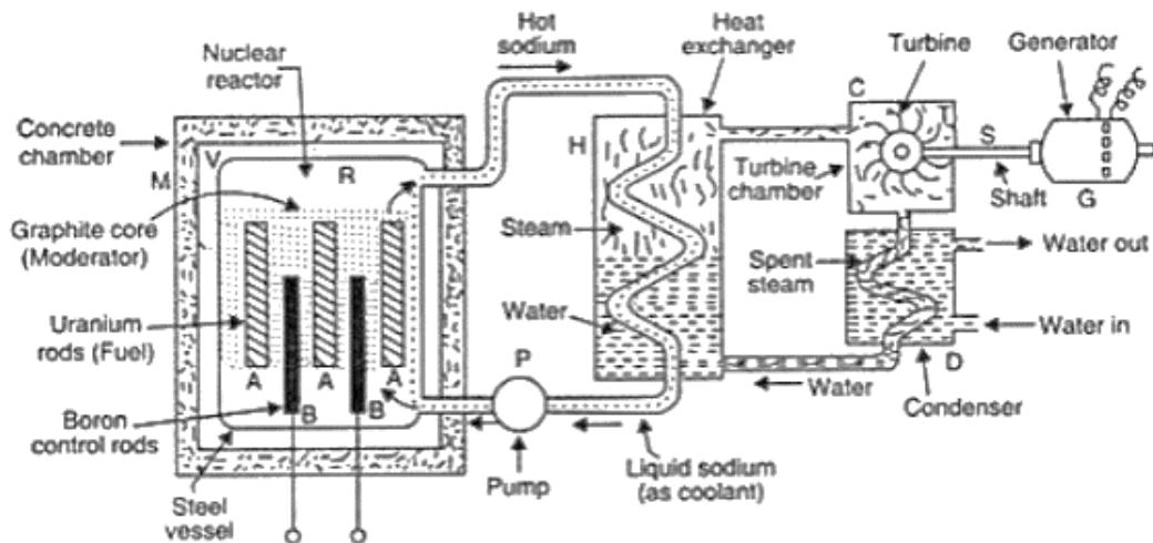
In a nuclear power plant, the fission of uranium- 235 is carried out in a reactor R. Uranium235 rods are inserted in a graphite core which acts as a moderator to slow down the neutrons. Boron rods B absorb excess neutrons and control the rate of reaction. Liquid sodium or carbon dioxide gas pumped continuously through pipes embedded in the reactor using a pump P is used as a 'coolant' to transfer the heat produced to the heat exchanger for converting water into steam. The hot steam at
