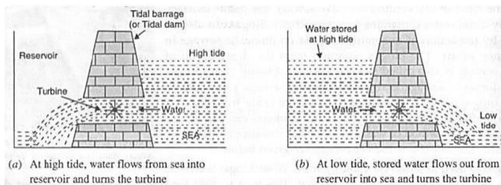
During high tide, when the level of water in the sea is high, seawater flows into the reservoir of the barrage and turns the turbines. The turbines then turn the generator to produce the electricity. And during the low tide, when the level of seawater is low,
