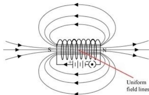
The magnetic field lines inside a current-carrying long straight solenoid are uniform.
