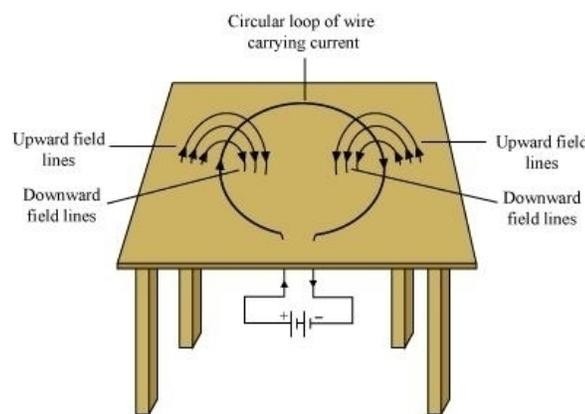
For the downward direction of current flowing in the circular loop, the direction of magnetic field lines will be as if they are emerging from the table outside the loop and merging in the table inside the loop. Similarly, for the upward direction of current flowing in the circular loop, the direction of magnetic field lines will be as if they are emerging from the table outside the loop and merging in the table inside the loop, as shown in the given figure.
