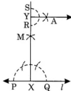
Step III: With  $P$  and  $Q$  as centers and a radius greater than  $PX$  draw two arcs to intersect each other at  $M$ .
